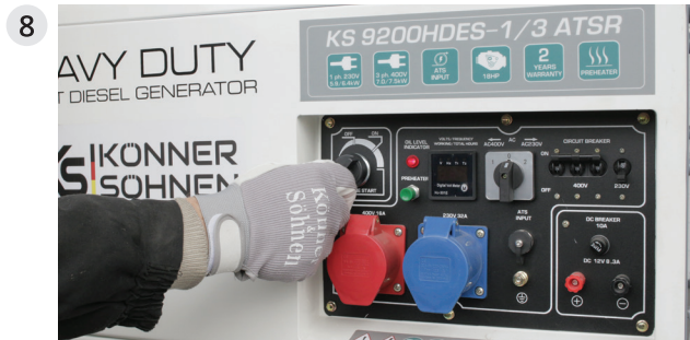
Turn the start key to "START" and hold it in this position for a few seconds. After 2-3 seconds, release the compression release lever without releasing the start key. After the engine starts, release the start key for it to return to "ON".
